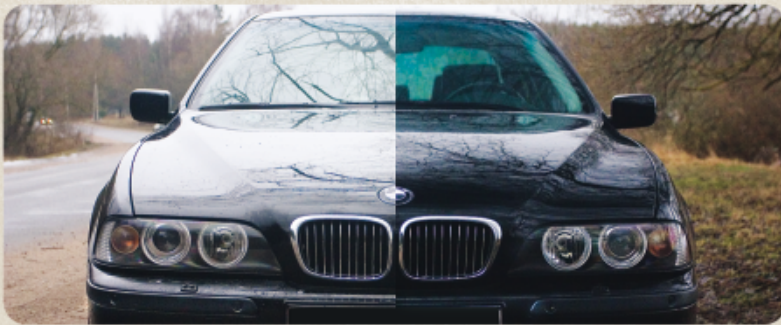
Observation in "Reflection" mode neutralizes or minimizes the dazzling effect of light reflected from non-metallic surfaces (water, snow, ice or glass).
