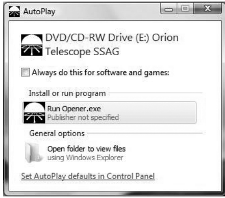
Figure 7. In Windows Vista the AutoPlay screen appears when you insert the CD-ROM into your computer. Select Run Opener.exe when prompted with this screen.
