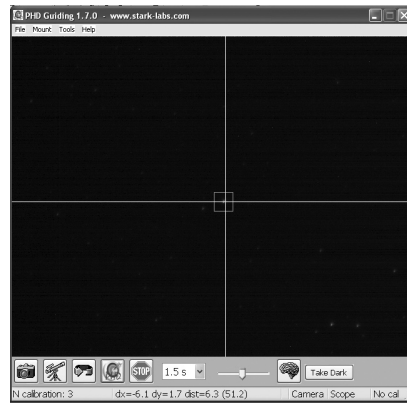
Figure 10. Yellow crosshairs appear once the calibration begins. The process is automatic. The crosshairs turn green when guiding begins.
