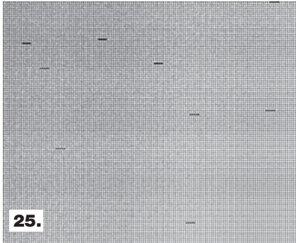
Figure 25. Readout artifacts similar to the ones shown here can occur if the camera readout speed is set too fast for your computer.
